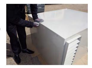
Slide the door panel 5 up under the top cover and fix using 3 x M6 X 12 set screws (12) at the base and 4 x M4 X 25 set screws (11) and 4 x nylon washers (14) at the sides. A single M4 X 16 set screw (13) fixes the door to the top cover.
