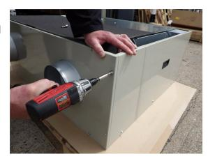
Place the top cover 1 over the housing panels and fix using 8 x M4 X 16 set screws (13) and 8 x nylon washers (11)
